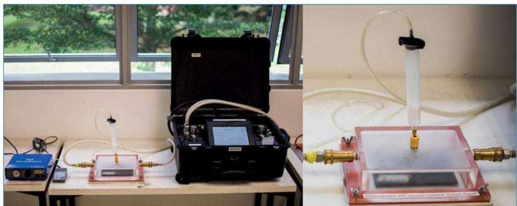
Fig. 1: Vacuum chamber with resin injection system for composite repair
