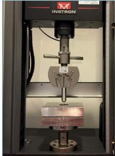
Fig. 6: Quasi-static indentation using a universal testing machine
