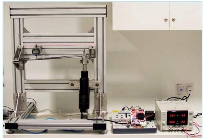
Fig. 7: Designed bending test rig for composite beams
