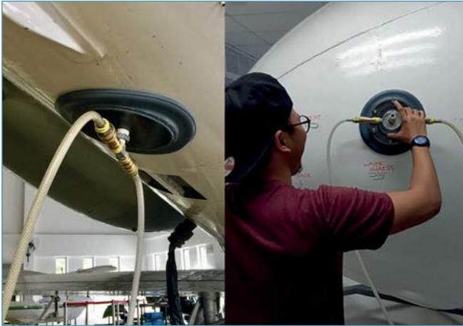
Fig. 2 & 3: Suction test on a composite aircraft fuselage and radome using a vacuum suction plate which will be adapted to the new vacuum chamber design
