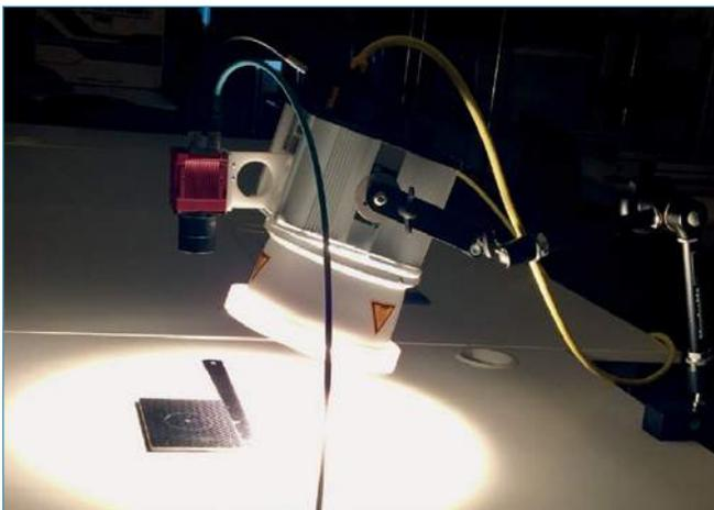
Fig. 5: NDT equipment- Infrared thermography from Automation Technology GmbH
