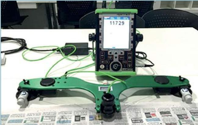
Fig. 4: NDT equipment- Ultrasonic flaw detector (Raptor) from NDT Systems, Inc
